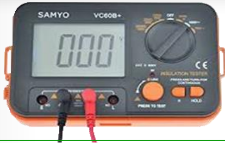
Insulation Resistance Test
